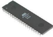
Figure 5: The AT89C51 Microcontroller
