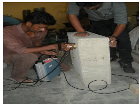
Fig 2. UPV on slab
